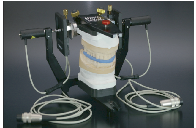
Fig 2 E-CPM with interposed model pair and working bite, which reproduces the previously recorded habitual occlusion.
