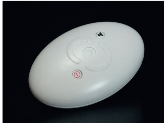
Fig 2 Receiving set with hidden USB connector to a PC (image courtesy of CMD-Centre Hamburg-Eppendorf)
