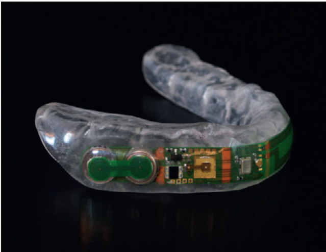
Fig 1 Michigan-type occlusal splint (modified according to Tanner) with integrated sensor and transmitter (prototype, image courtesy of CMD-Centre Hamburg-Eppendorf).
