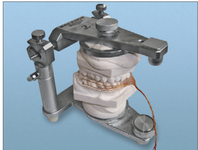
Fig 4 Semi-adjustable articulator with situation models, occlusal splint and sensor prototype, here still without the radio transmitter (image courtesy of Clauss, TU-Munich).
